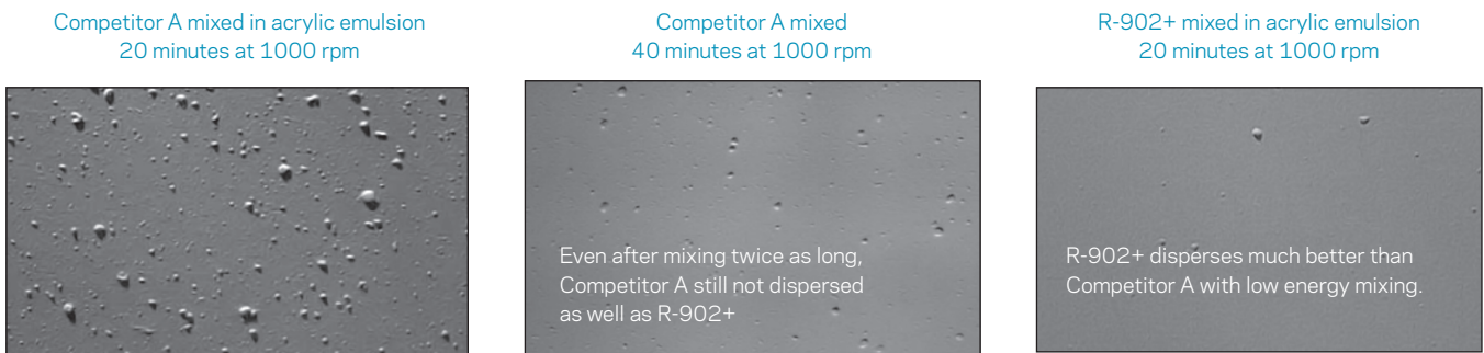
Figure 4: Ti-Pure™ R-902+ Allows Waterborne Dispersion Time and Energy Savings
