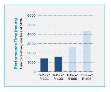
The performance time data of PVC parts comprising Ti-Pure™ TiO₂ materials and additive packages typical for NA exterior PVC demonstrates how PVC parts exposed to exterior weathering simulation with TiO₂ grades specially designed for durability and longevity (R-960 and R-105) deliver extended performance time.
